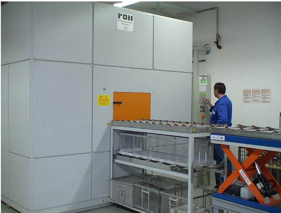
Picture 1: Loading of the working chamber by means of the roller conveyor
