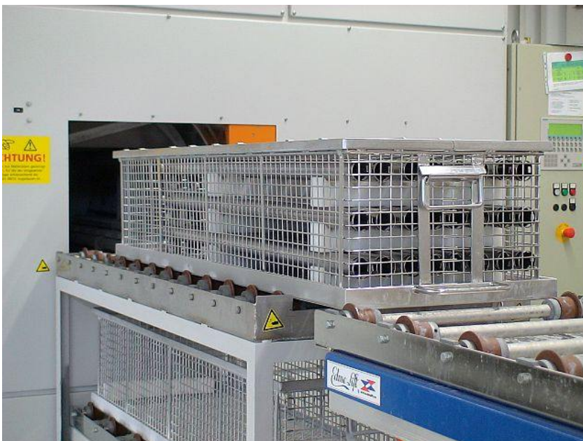
Picture 2: Pump pipes in a special basket prior to cleaning
